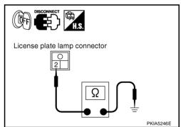
Check continuity between rear combination lamp harness connector and ground.
