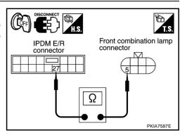
Check continuity between IPDM E/R harness connector E7 terminal 20 (LG) and front combination lamp RH harness connector E24 terminal 6 (LG).
