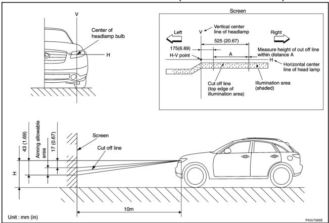
If the vehicle front body has been repaired and/or headlamp assembly has been replaced, check aiming. Use the aiming chart shown in the figure.
