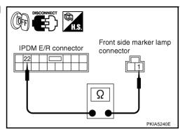
4. Check continuity between IPDM E/R harness connector and clearance lamp harness connector.
