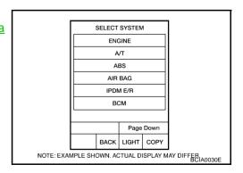
Select the desired part to be diagnosed on "SELECT DIAG MODE" screen.
